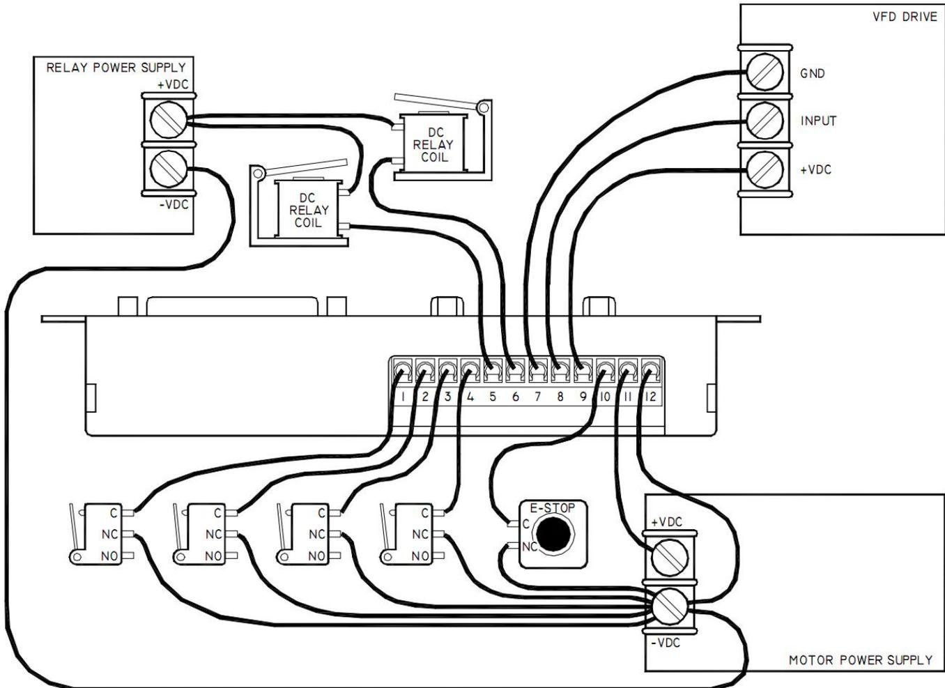
Please note that all connections shown above are optional except for the power supply and E-Stop switch. A few frequently asked questions for wiring are below:
